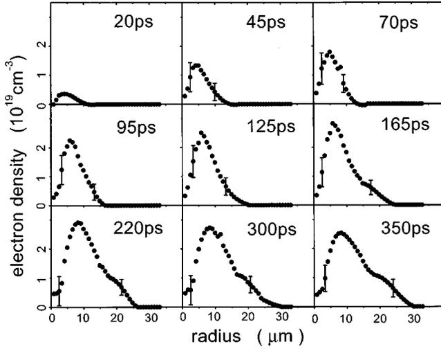
FIG. 3. Electron density profiles determined from interferometry. Pump pulse  $\lambda=1064$  nm, 100 ps, peak intensity  $2.5 \times 10^{12}$  W/cm<sup>2</sup>. The time  $t=0$  corresponds to a peak electron density of  $5 \times 10^{17}$  cm<sup>-3</sup>, representing the minimum detectable phase shift. The vertical bars represent the statistical standard deviation of profiles derived from individual phase lineouts.
