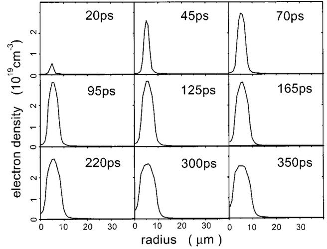
FIG. 4. Electron density profiles from simulation. The time  $t=0$  is set from the appearance of a peak electron density of  $5 \times 10^{17}$  cm<sup>-3</sup>.
