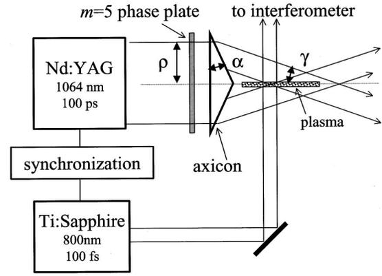
FIG. 1. Experimental arrangement, showing synchronization of Nd:YAG and Ti:sapphire laser systems, hollow beam optics, and interferometer setup.
