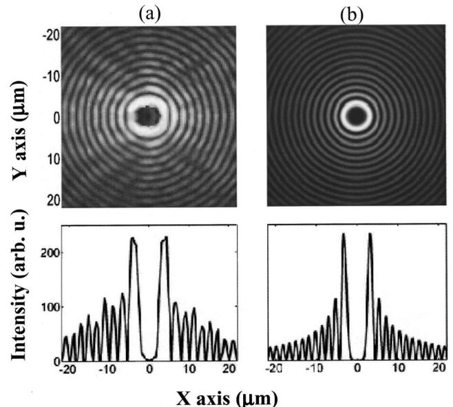
FIG. 2. (a) Image and lineout of focal region of  $m=5$  phase plate and axicon combination for  $\lambda = 1064 \text{ nm}$ ; (b) Theoretical plot and lineout for  $|J_5|^2$  for  $\gamma = 19^\circ$  and  $\lambda = 1064 \text{ nm}$ .
